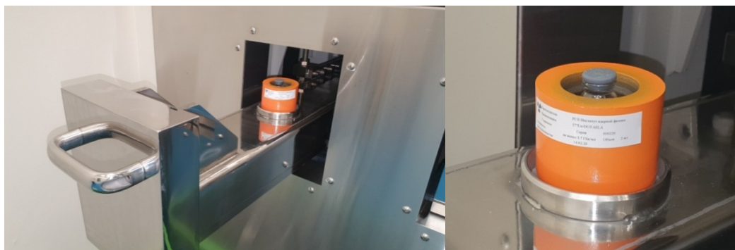
Figure 35 - Unloading the drug container from the hot chamber
