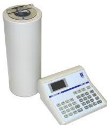
Figure 11 - Capintec CRC - 25R Dose Calibrator
